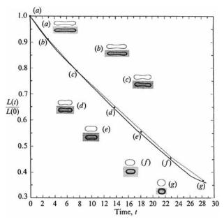
FIGURE 11. Quantitative comparison of numerical (solid curve) and experimental results (dotted curve) for relaxation of an initially extended droplet in a quiescent fluid;  $\lambda = 0.45$  – a test of the constant-interfacial-tension boundary condition. Still photographs and corresponding numerically generated shapes are shown.
