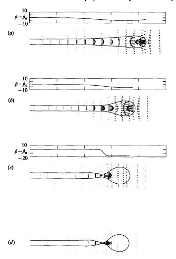
FIGURE 6. Velocity and pressure fields for a relaxing drop in an otherwise quiescent fluid;  $\lambda = 0.1$ . The pressure field  $\hat{p} - \hat{p}_0$  shown is the droplet pressure along the centreline (r = 0) and is measured with respect to zero at the droplet centre (r, z) = (0, 0). (a) t = 0; (b) 22.40; (c) 28.97; (d) 32.64.
