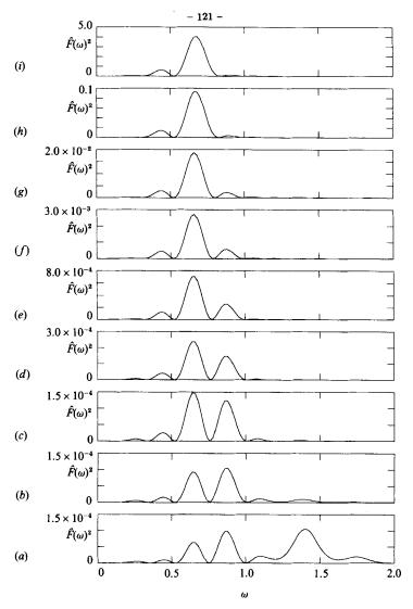
FIGURE 14. Evolution of the Fourier spectrum of the disturbance on the central cylindrical region of the drop. Fourier decomposition calculated using equation (5) with l=20. (a) t=0; (b) 10.0; (c) 20.0; (d) 30.0; (e) 50.0; (f) 73.0; (g) 104.6; (h) 170.6; (i) 194.6. Modes that are stable in the linear stability theory are  $\omega > 1$ . All  $0 < \omega < 1$  are unstable according to the linear theory. Notice that the dominant mode initially is a linearly stable mode and it rapidly decays.
