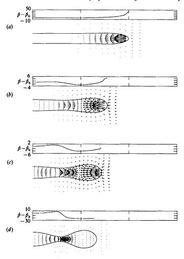
FIGURE 10. Velocity and pressure fields for a relaxing drop in an otherwise quiescent fluid;  $\lambda = 0.01$ . The pressure field  $\hat{p} - \hat{p}_0$  shown is the droplet pressure along the centreline (r = 0) and is measured with respect to zero at the droplet centre (r, z) = (0, 0). (a) t = 7.54; (b) 18.54; (c) 27.74; (d) 29.74.
