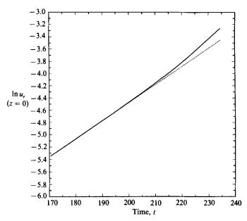
FIGURE 16.  $\ln u_r(z=0)$  versus t. The solid line represents the numerical calculations. The dashed line is a straight line with the same initial slope. The slope of this line yields a growth rate of  $\gamma=0.030$  which is in good agreement with the prediction of the linear theory based on the dominant mode,  $\gamma(0.66)=0.033$ . At later times the interface evolves more rapidly than the linear theory predicts.
