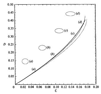
FIGURE 2. Drop deformation in a steady axisymmetric extensional flow: D  $vs. \mathbb{C}$ ;  $\lambda = 0.1$ . The solid line represents the numerical simulation and the dashed lines are the predictions of the small-deformation theory of Barthes-Biesel & Acrivos (1973). The short-dashed line denotes the  $O(\mathbb{C})$  result and the long-dashed line the  $O(\mathbb{C}^2)$  result. Several numerically generated steady shapes are included.
